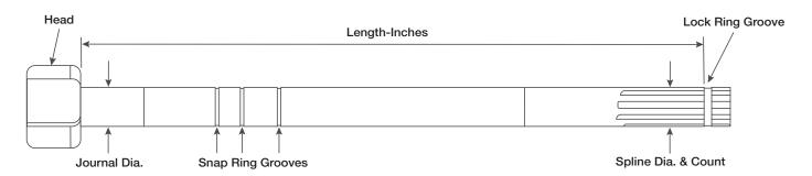
Measure from under the cam shaft head to the first lock ring groove. (If two lock ring grooves, measure from the groove Length:
